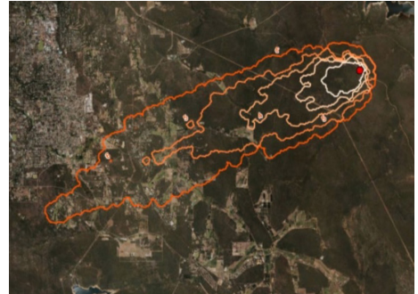
A fire spread prediction map showing showing isochrones - contours outlining the burnt area at equal time intervals. The ignition point is marked by a red dot. Credit: Jackson Parker, DFES (WA).
